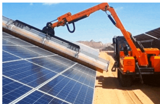
LAVAGGIO PANNELLI SOLARI SOLAR PANEL WASHING
